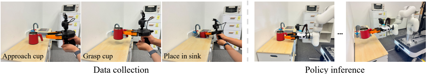
Fig. 5. The task involves robotic manipulation to grasp a cup and place it into a sink. The first three images depict a human operator utilizing the Fast-UMI interface-mediated manipulation device to collect demonstration data. The subsequent two images show the robot executing an inferred action policy, trained on the collected data using the ACT algorithm.
